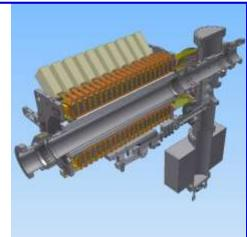
**Step 2**: Formation of the short ion bunches at presence of cooling: <u>RF-2 (100 kV, 4 cavities)</u> from coasting beam to => 22<sup>nd</sup> harmonics
