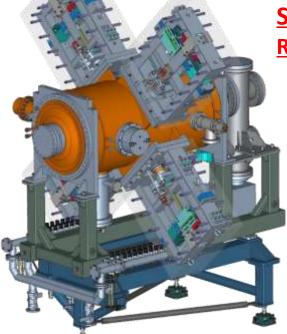
Step 3: Interception of the short ion bunches into separatrix of 66<sup>th</sup> harmonics RF-3 (1MV, 8 cavities).
