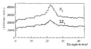
Fig. 11. Photon yield and radiated energy from a 1 mm thick tungsten crystal versus tilt angle between (111) axis and electron beam for an incident energy of 2 GeV. Rotation axis is the vertical one, the collimation angle is 1 mrad (from Ref. [14]). Both curves are represented in arbitrary units for the vertical scale.
