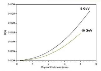
Fig. 3. Total energy deposited in the radiator: ratio  $Q(x) - E_{dep}/E$  for E = 5 and 10 GeV.
