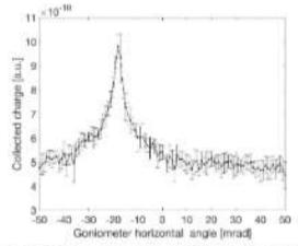
Figure 4: Rocking curve measured by the diamond sensor. Collected charge by the diamond sensor is plotted as a function of the goniometer rotational angle.
