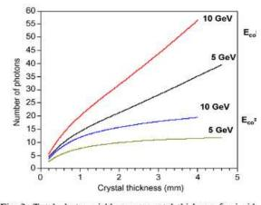
Fig. 2. Total photon yield versus crystal thickness for incide energies of 5 GeV and 10 GeV, E<sub>cut off</sub> – 5 MeV: upper curve 50 MeV: lower curves.
