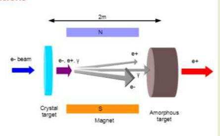
Figure 5.1: Hybrid scheme using crystal and granular target for ILC.
