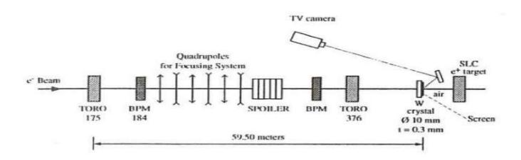
Figure 3: The SLC experimental set-up
