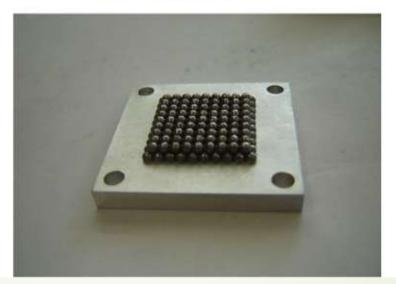
With respect to bulk targets a granular target made of small spheres ( $\phi$ ~ 1 mm) presents better heat dissipation
