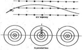
Figure 10: Axial channeling on a Si < 111 > crystal.
