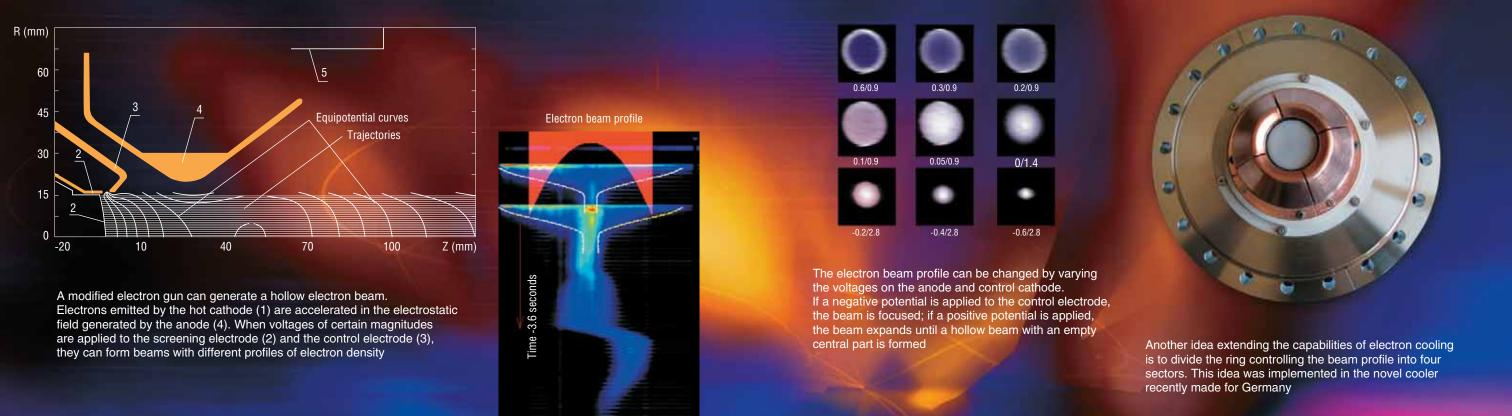
electron beam so that the electron density had the maximum value on the beam periphery, and the dense ion beam was accumulated in the central part with a small number of electrons.
