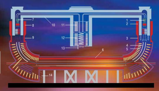
The electron cooler has a fairly simple structure. The electron beam is generated by an electron gun having a specially shaped cathode. After that, the beam is accelerated and directed to the channel of the main accelerator with the help of a deflecting system. Then the electron beam is directed outward (with the help of the same deflecting system), and electrons are collected in a collector
