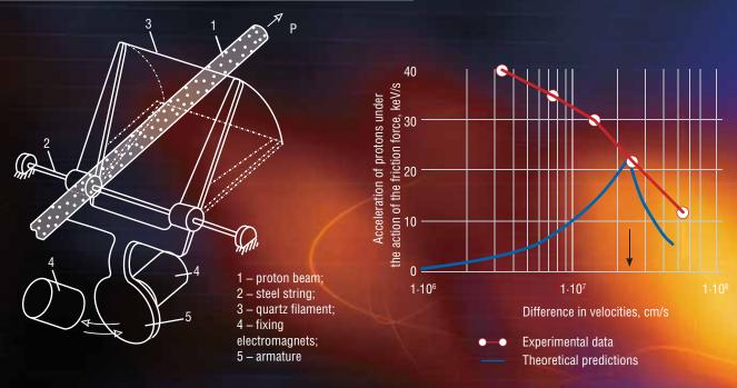
A simple but effective device for measuring the profile of the beam of accelerated protons. A quartz filament with a cross-sectional area of several microns crosses the beam. By measuring the intensity of particles scattered by the wire, One can perform precision measurements of the density distribution of protons over the beam cross section
